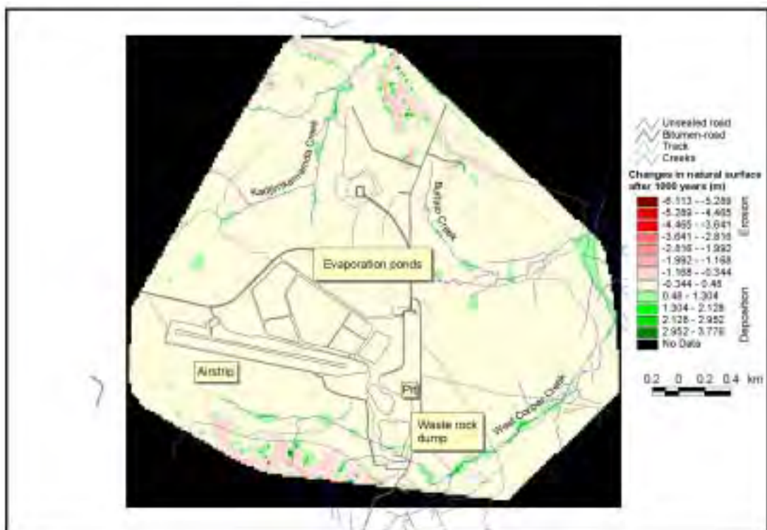
Figure 9 Erosion and deposition on the landform at 1000 y under natural surface conditions.
