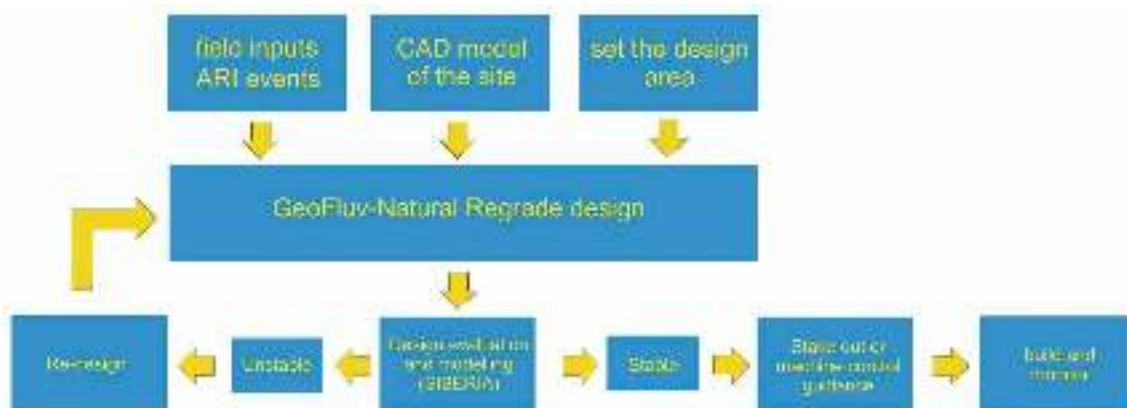
Fig. 4. Diagram showing a GeoFluv design – SIBERIA modelling for maximizing landform stability in mine rehabilitation.
